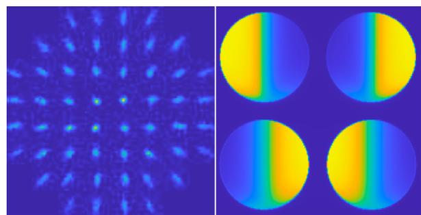
SHWFS spot pattern for a laser guide star<sup>1</sup> and Intensities in the detector of the PyWFS for a flat wavefront<sup>2</sup>.
