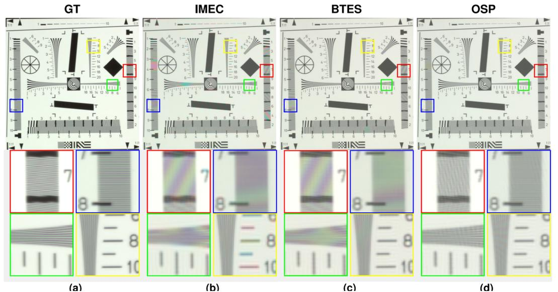
Comparison of Zipper effect and color distortion between three MSFAs. The chart scene of TokyoTech has a spatial resolution of  $736 \times 736$  and 16 spectral bands, and the reconstruction algorithm is ItNCD.
