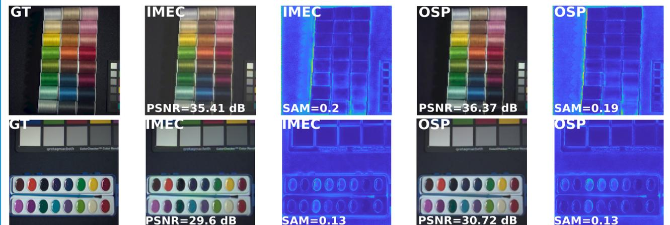
Comparison between MSFAs, including spectral response of the Ximea camera with spatial resolution  $256 \times 256$  and spectral resolution 16.
