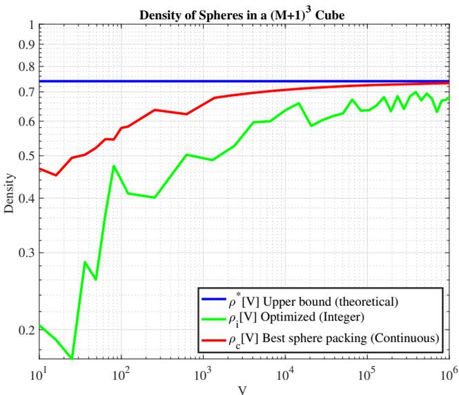
Fig. 2. SP density comparison for different dimensions; (blue line) theoretical upper bound where the cubic container has size  $(M + 1)^3$ , and the total number of spheres is  $V = MN$ ; (red line) best known optimal sphere packing without the MSFA restriction; (green line) OSP density with MSFA restriction.
