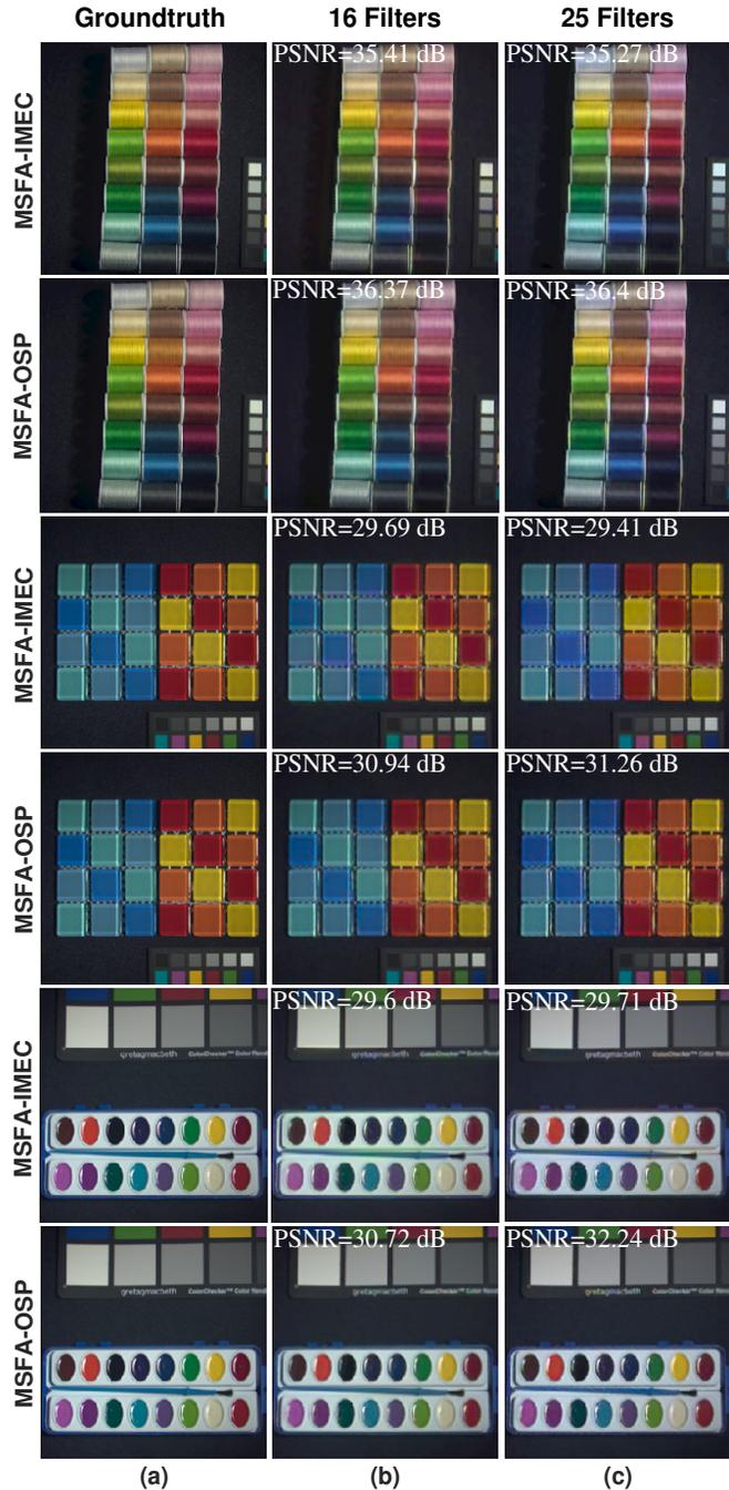
Fig. 9. Comparison of spatial fidelity between MSFA-IMEC and MSFA-OSP using real filters. For the experiment, the dichroic filters are replaced by the spectral response of the IMEC camera, and the reconstruction algorithm is TRevSCI. The first column in Fig. 9(a) shows the RGB groundtruth of three scenes thread spools, glass tiles, and paints. The second column in Fig. 9(b) and third column in Fig. 9(c) depict two different filter numbers,  $L = 16$  and  $L = 25$ .
