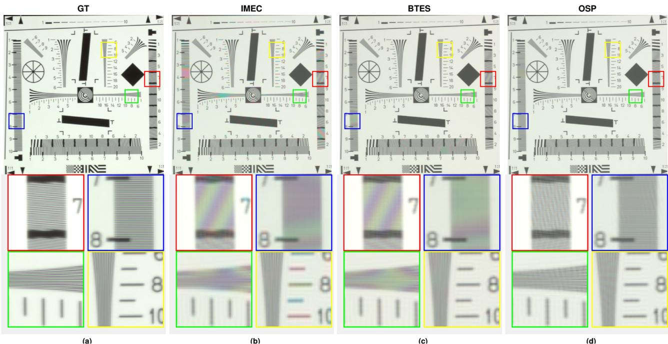
Fig. 6. Zipper effect and color distortion comparison between three MSFAs. The chart scene of Tokyotech [36] has a spatial resolution of  $736 \times 736$  and 16 spectral bands, and the reconstruction algorithm is ItNCD, where (a) is the groundtruth (b) is IMEC, (c) is BTES, and (d) our proposed OSP approach. Four squares show zoomed versions of the scene; note the significant zipper effect and color artifacts in state-of-the-art patterns.
