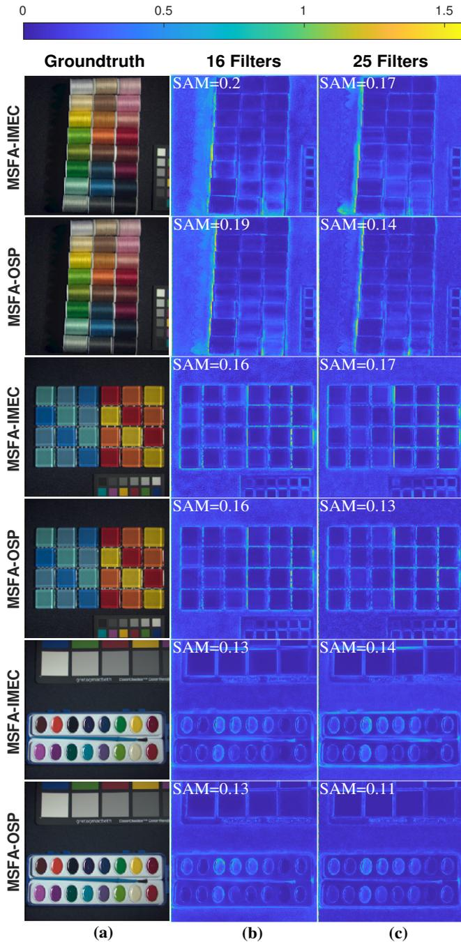
Fig. 10. A comparison of spectral similarity between MSFA-IMEC and MSFA-OSP using real filters means that the dichroic filters are changed for the spectral response of the IMEC camera, and the reconstruction algorithm is TRevSCI. The first column of Fig. 10(a) depicts the groundtruth of the thread spools, glass tiles, and paints of three scenes. The second Fig. 10(b), and third Fig. 10(c) columns show the spectral similarity of IMEC and OSP with 16 and 25 filters, respectively.
